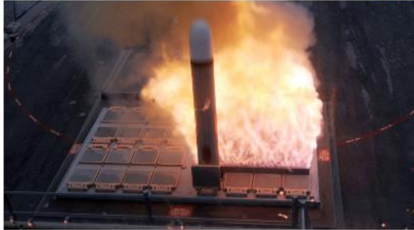
A Tomahawk missile being launched from the Mark 41 Vertical Launching System aboard United States Navy destroyer USS Farragut. File photo. © the United States Navy / Wikipedia
