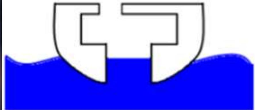
B) An open moon pool at the waterline, in a ship or floating structure
