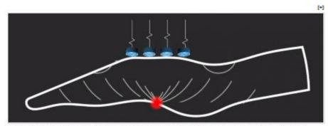
The SkinHaptics device sends ultrasound waves through the hand, focused at a precise point on the palm. (credit: Sri Subramanian / University of Sussex)
