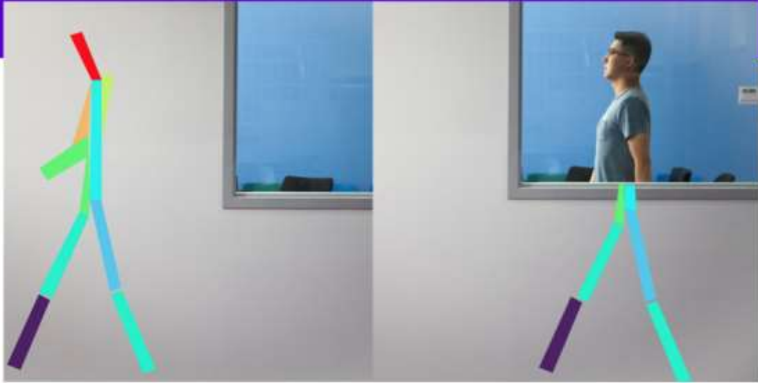
Using wireless signals, RF-Pose could serve as a health care system to monitor patients' movements from the other side of a wall. MIT CSAIL
