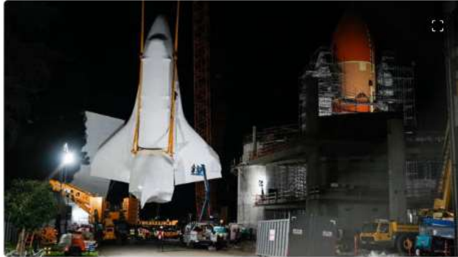
The Endeavour orbiter was hoisted atop an external tank and two solid boosters. © Photo: Ashley Landis (AP)
